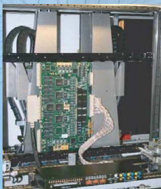
Flyscan inserts the Flying Probe tester into the JTAG chain
